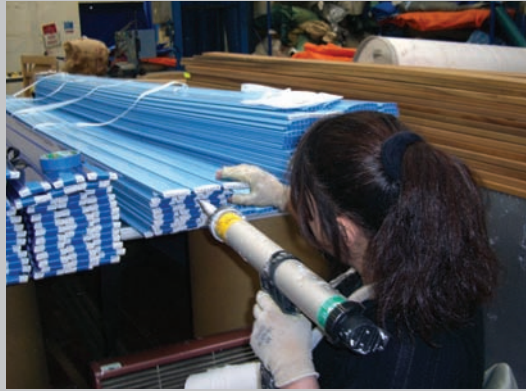
End caps being siliconed using pneumatic pressure silicone guns.
