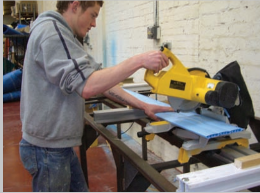
Slats being cut to length on our own design cutting machine.
